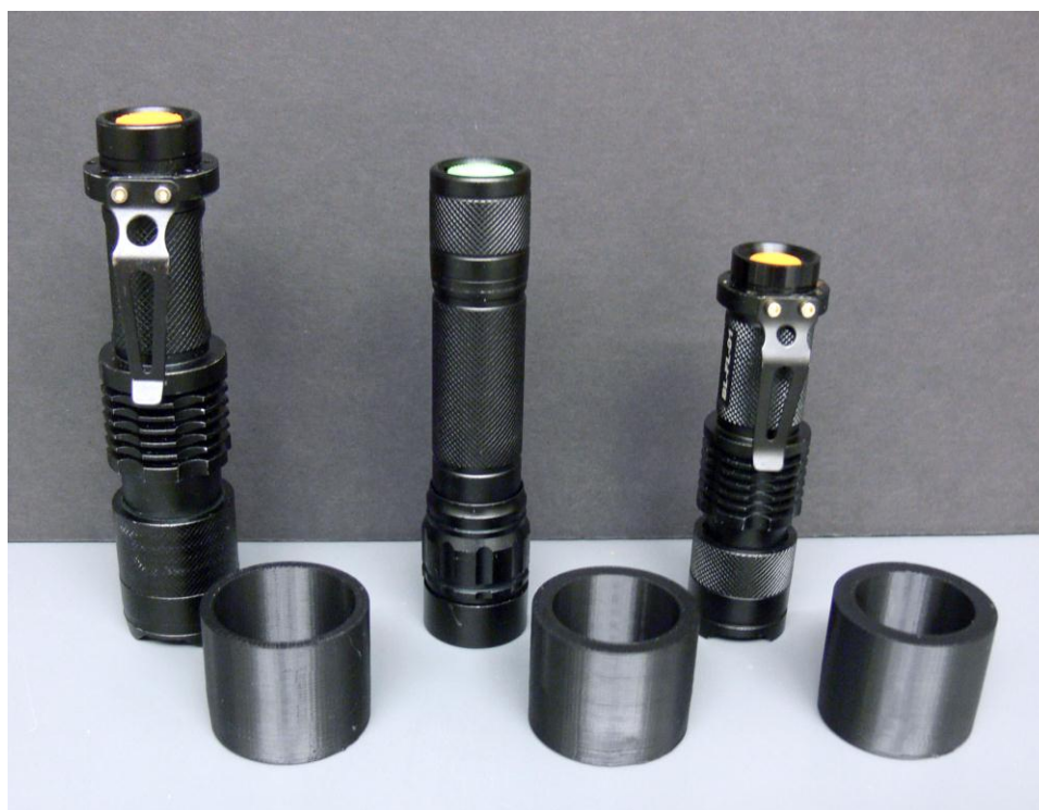
155 Figure S1-5. Adapters for three small tactical LED flashlights that we use with the OPN Fluorometer. From left to right, the UltraFire, SkyWolfEye, and GeakLight flashlights. Readers can place these adapters into the tube for an Outlite WT03 flashlight, which should cut down on 3D printing costs.
