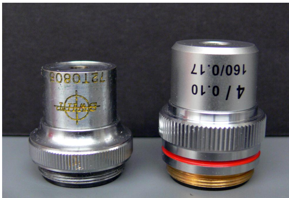
Figure S1-2. Microscope objective lenses (4x) that we use with our OPN Fluorometers. A used 4x objective lens from a Carlsan microscope that we purchased on eBay (left). A new 4x objective lens made by AM Scope (SKU No. A4X-V300; right).
