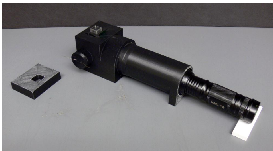
Figure S1-1. The 3D-printed version of the OPN Fluorometer, which holds an Outlite WT03 tactical LED flashlight. Note that we used a small piece of white PVC board in this set-up (lower right) to prop up the handle of the flashlight and, thus, level the beam.
