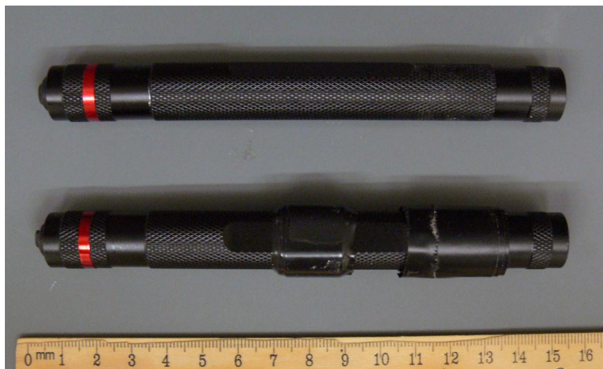
115 Figure S4-5. Wrapping a Coast G20 LED inspection light with electrical tape, so that it will fit snugly into a \frac{3}{4} -inch PVC tube.
