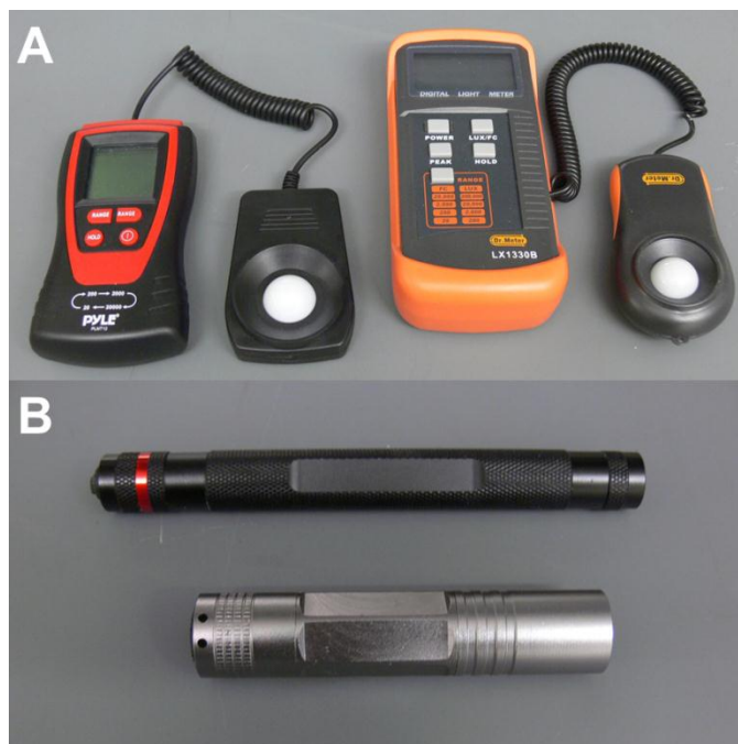
Figure S4-1. The commercial light meters and LED flashlights that we use with our OPN Colorimeters. (A) Pyle PLMT12 (left) and Dr. Meter LX1330B (right) light meters. (B) Coast G20 LED inspection light (top) and 35-lumen LED keychain light (bottom).
