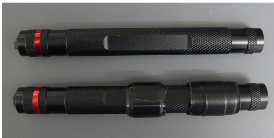
Figure S4-6. Wrapping a Coast G20 flashlight with electrical tape in two places, so that it will fit smoothly into a ¾-inch PVC tube.
