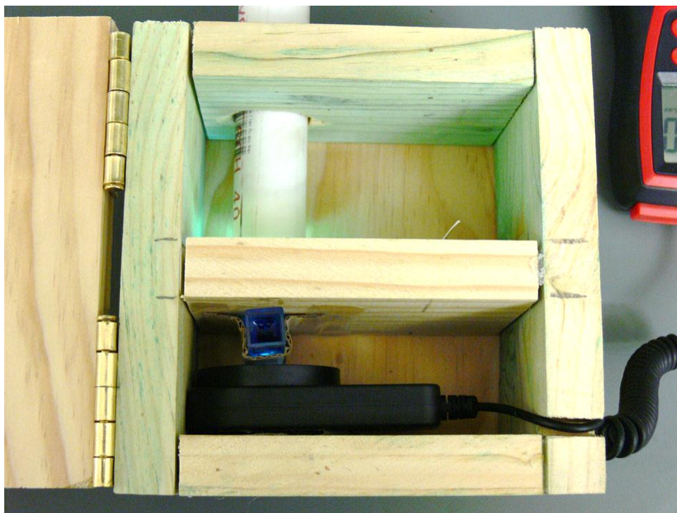
Figure S4-4 Placing the cuvette holder in the back chamber of the OPN Colorimeter. Note that we used a piece of cardboard as our holder in this design.
