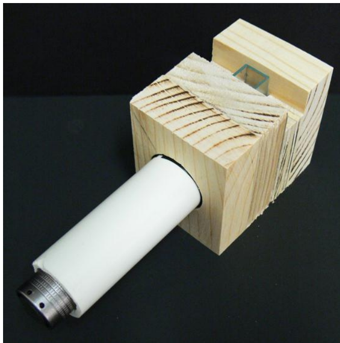
Figure S4-9. The assembled pieces for a wooden version of the OPN Colorimeter, which can hold a light dependent resistor (LDR), without the lid in place.
