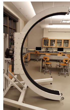
Figure 1B. SoLoArc in Elevation configuration: The device rotated into vertical position. The participant would be seated with their head at the convergence focal point directly between the -90° and +90° speaker.
