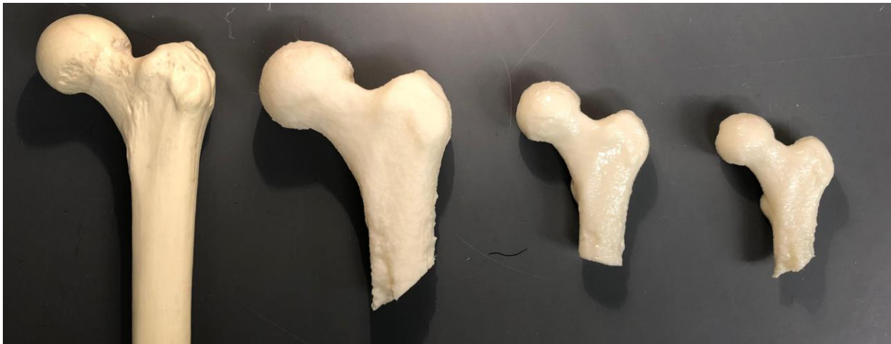
Figure 7: This image shows the preserved level of detail between scaled photogrammetry meshes and prints.
