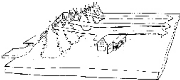
Figure 24—Evergreens protect a building from dust and cold by reducing windspeeds (from Sand 1993).
