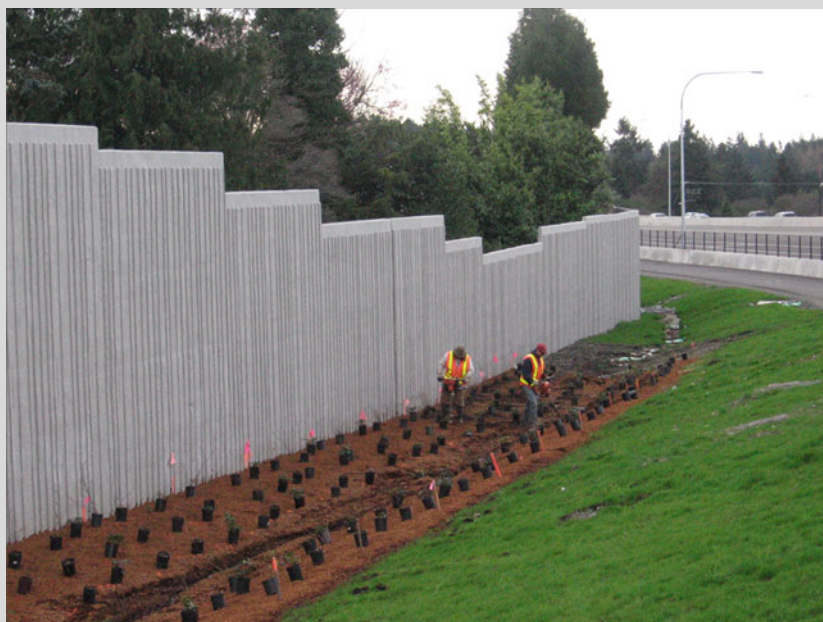
Fig. 9.7 Installing an experiment to test plant response to compost amendments along a highway right of way outside of Tacoma, WA (Data from this study is shown in Table 9.5. Photo credit: Andy Bary)
